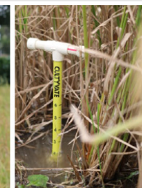
Functioning of water level measuring tool
